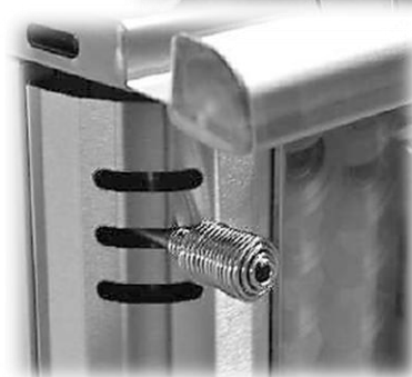
closed flue gas deflector (17)
